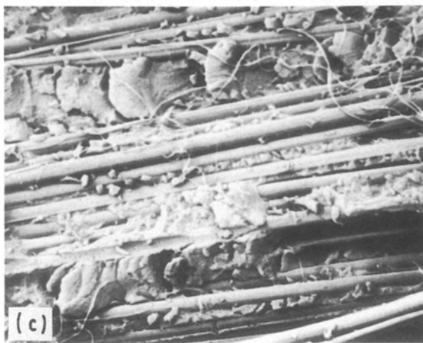
Figure 30 Temperature dependence of tensile fracture surface (L), of ARALL 4 laminates showing interface–matrix shear failure and fibre pull-out/fibrillation: (a) -65^{\circ}\text{F} ( -54^{\circ}\text{C} ), (b) 75^{\circ}\text{F} ( 24^{\circ}\text{C} ), (c) 400^{\circ}\text{F} ( 204^{\circ}\text{C} ). \times 350
