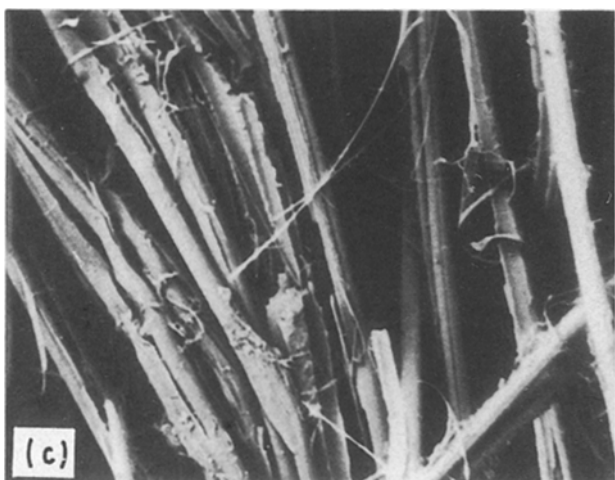
Figure 32 Temperature dependence of tensile fracture surface (T) of ARALL 4 laminates showing fibre and matrix separation at the interface and fibre splitting: (a) -65^{\circ}\text{F} ( -54^{\circ}\text{C} ), (b) 75^{\circ}\text{F} ( 24^{\circ}\text{C} ), (c) 400^{\circ}\text{F} ( 204^{\circ}\text{C} ). \times 350
